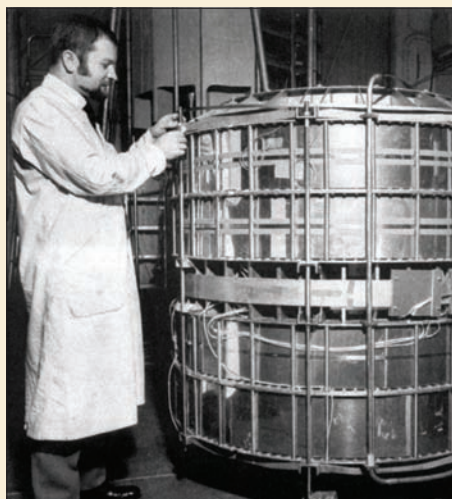
The large superconducting coil (BIM) being operated at Saclay to gain experience in superconductivity techniques.
