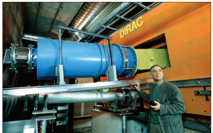
A general view of the downstream part of the DIRAC experiment (upper image) beyond the magnet (orange), with the yellow boxes of the Cherenkov counters in the foreground. The lower image shows the section between the beam shielding and the magnet, with the vacuum chamber (blue), the beginning of the flat chamber (yellow) and the magnetic screen (orange) in front of the magnet. The beam pipe for the primary protons (silver) lies beneath the blue vacuum chamber.
