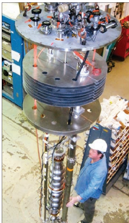
Cornell's first ERL cavity during its vertical test showing the required small energy loss. (Image credit: Cornell/LEPP.)
